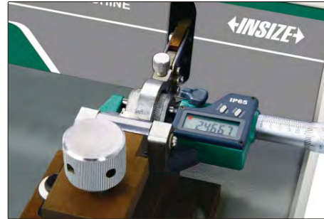
lapping measuring surfaces of outside micrometer
