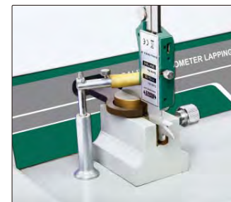
lapping measuring surfaces of caliper lower jaws
