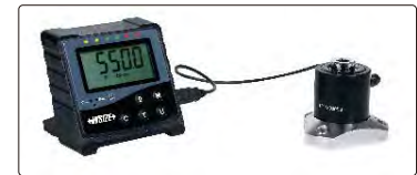
digital torque tester (optional)
