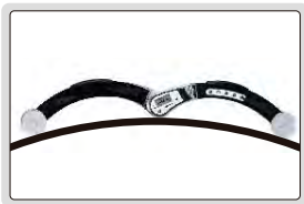
external diameter measurement
