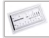
plastic calibration rule (included, graduation 1mm)
